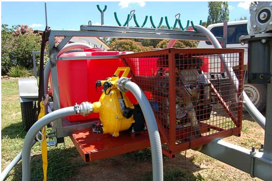
Figure 5: The front end of the slave trailer. A 20 HP air-cooled four-stroke motor (right, in protective mesh cage) powers a fire-fighting pump (yellow) that can be used to move ballast water between the prime mover and the ballast tanks on the trailers (red). The motor also delivers exhaust gas to the euthanasia system. Pic by C. Tidemann.
