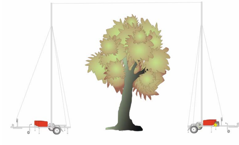
A trailer-mounted system for catching and euthanasing roosting Mynas
